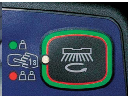
Raise, lower or even double the brush pressure right from the dashboard for even more cleaning power.
