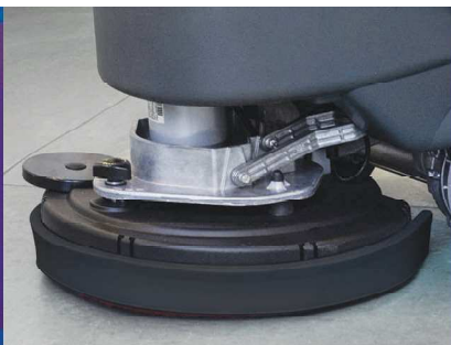
Optional splash guard keeps water in the path of the squeegee even at the fastest operation speeds.
